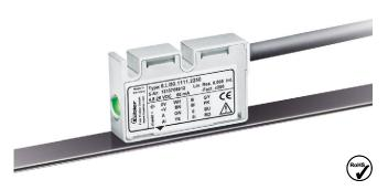
The non-contact incremental magnetic linear measurement system Limes LI50 / B2 - made up of the sensor head LI50 and of the magnetic band B2 - reaches a resolution up to 5  $\mu m$  with a maximum distance of 2 mm between the sensor and the band.
