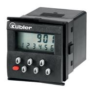
Type 901 is a simple battery-powered preset pulse counter/timer with 12 ... 250 V AC/DC count and reset inputs or with NPN input. The 6-digit, 2-line LCD display shows the current count value, the preset value, the relay state and the active time measurement.
